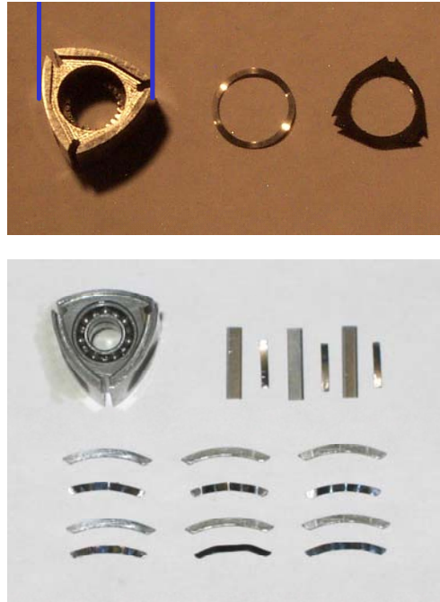
Figure 2. 1-pc. (top) and 3 pc. (bottom) Face (or side seals). Springs for each design are also shown.
