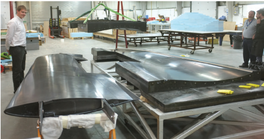
(Left) A completed wing assembly and, behind, the substantial mould/jig.
