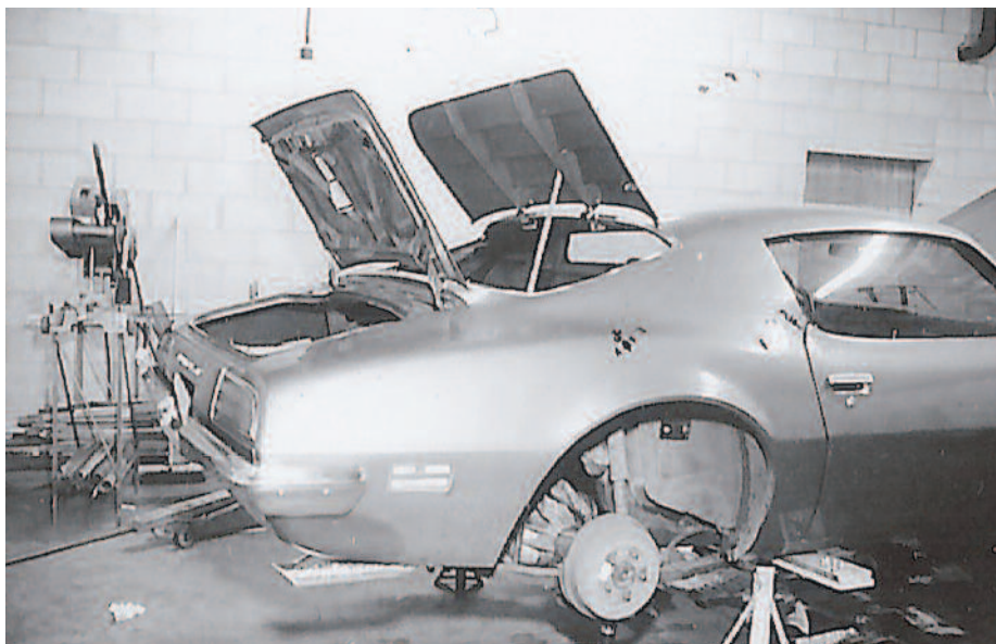
Interestingly, the location of the engine allowed for the stock trunk and fuel tank to be retained. A louvered hatch replaced the rear window. Note the Frankland differential located just inside of the right rear leaf spring. The location of the transaxle necessitated an offset differential location.
