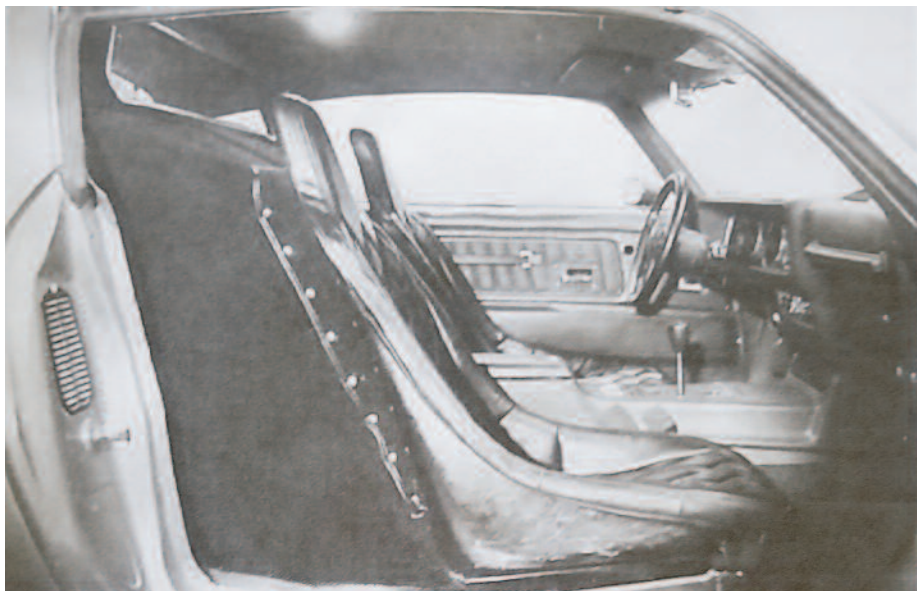
The engine encroached heavily into the Firebird's interior, restricting legroom to a certain extent. Thin-shell fiberglass seats were used to maximize the room that was left and the wheelbase was also extended one inch to help in that area.
