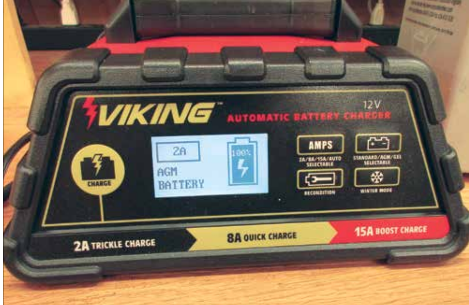
The HF battery charger confirming that it was using the AGM (Advanced Glass Mat) battery regimen for this battery.
