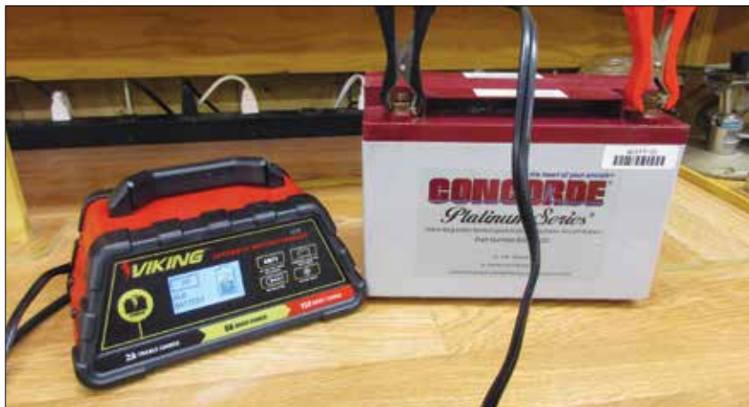
The Harbor Freight battery charger hooked up to the dead Concorde battery out of my '58 Cessna 182.
